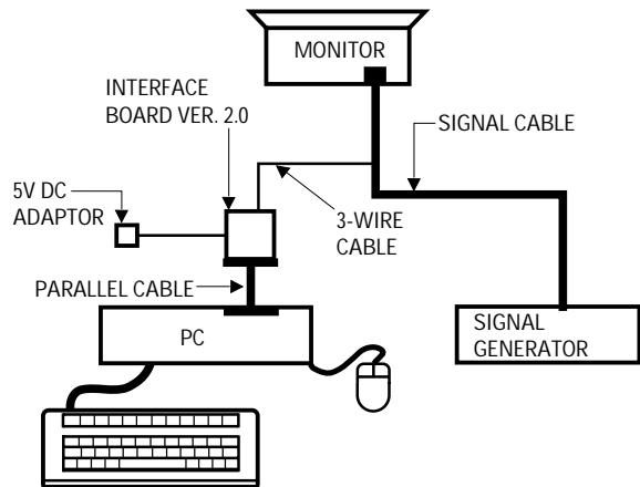
Figure 4-1. Setup 1, With Signal Generator
